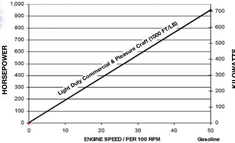
**Example:** For a pleasure craft boat with a gasoline engine, the Liberty Series delivers 950 HP at 5000 RPM.
